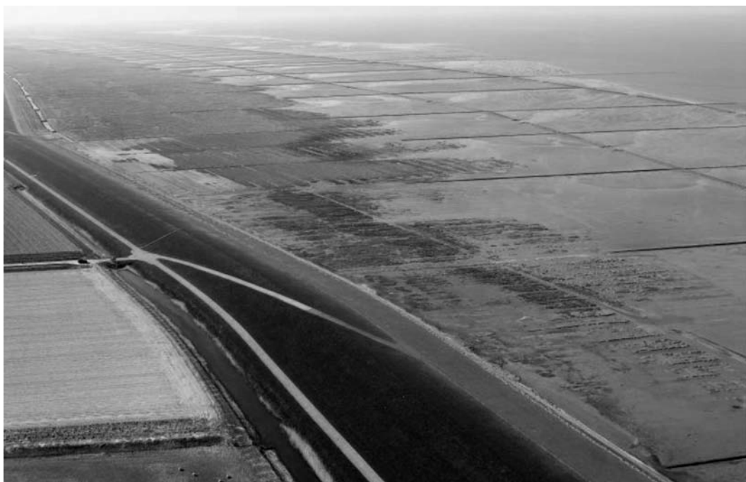
Figure 8.9 Extensive salt marshes with brushwood dams along a dike bordering the Dutch Wadden Sea. ( https://beeldbank.rws.nl , Rijkswaterstaat.)
